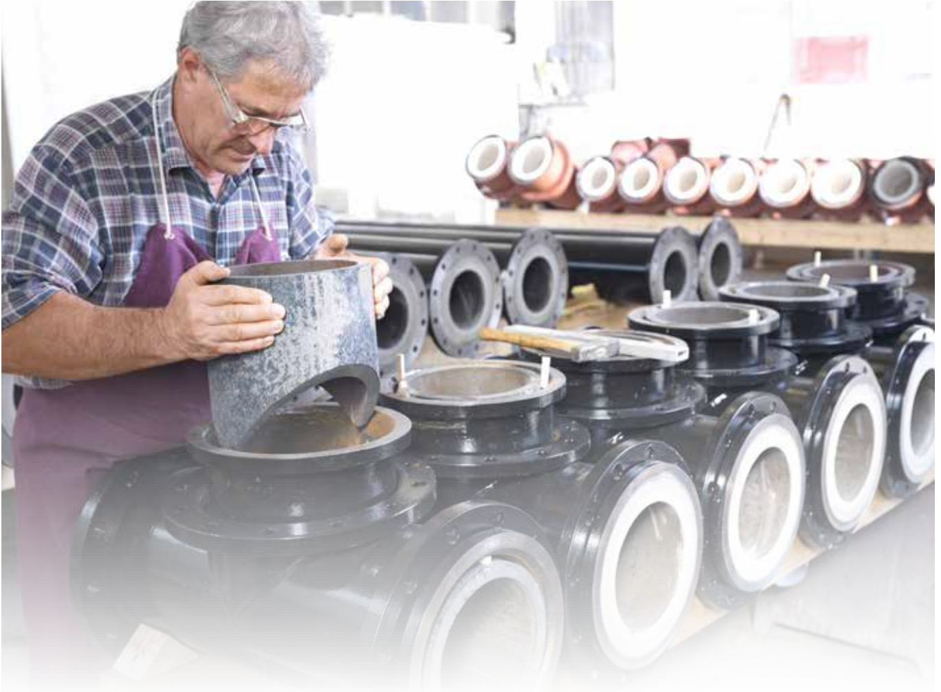
Assembly of the lining with cylinders
