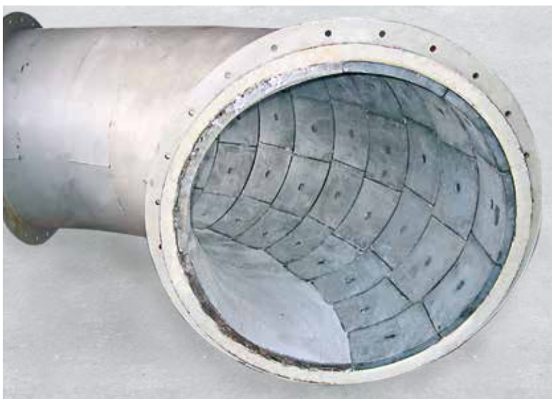
Kalenborn pipe bends for a plastic waste shredder plant: combination of KALCAST hard castings and KALCRET hard compound
