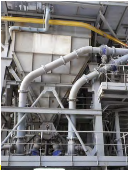
Pneumatic KALOCER transfer line with moulded components for conveying alternative fuel (demolition wood with sand particles) to a furnace, cross-section 203 mm.
