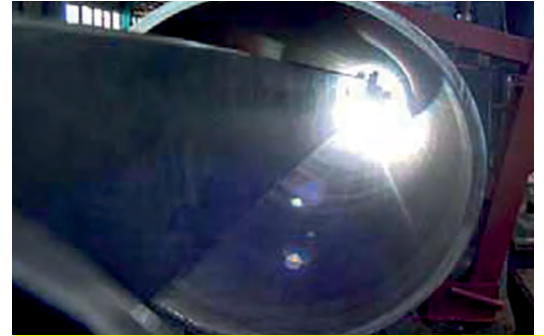
Automatic welding machine for lining the interior of a pipe Hard-facing of workpieces with cored wires and electrodes Pipe component weld joint
