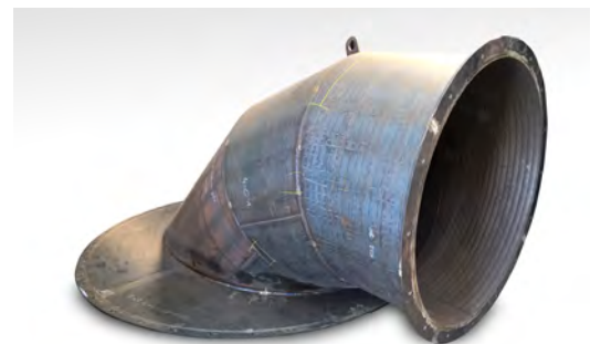
Pipe bends lined with KALMETALL in a de-dusting system application, the inner diameter is 400 mm, the system thickness is 8 + 5 mm.
