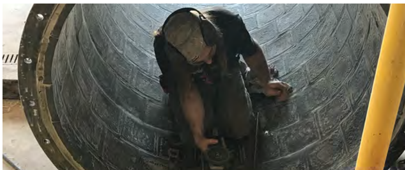
Kalenborn special ducts and bends for a biosolids recycling plant: straight ABRESIST ducts and bends with KALOCER and KALCRET
