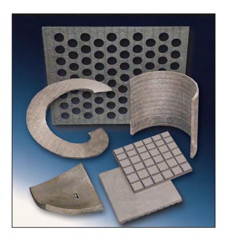
KALMETALL® is a combination of a strong steel base and a hard overlay welded chromium carbide protective layer that resists abrasion, impact and high temperatures. The base consists of standard carbon steel or alloy plates designed to suit your specific application. The protective layer is composed of a C-Cr-Fe system with primary chromium carbides and is an integral part of the structure.
