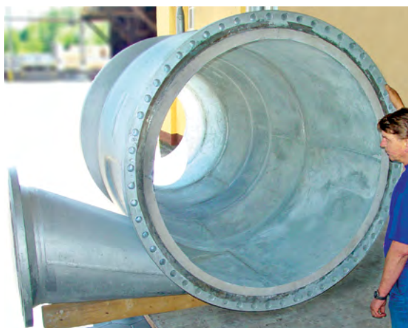
1,200 mm diameter KALSICA cyclones guarantee reliable operation: the system separates silicon sand at temperatures up to 300 °C / 572 °F
