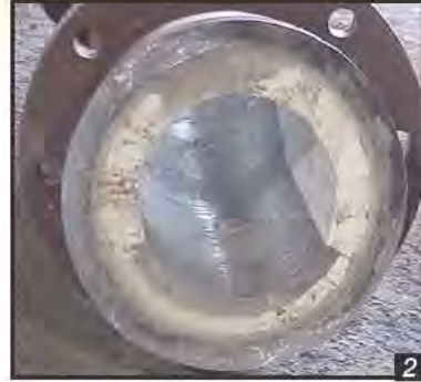
1. Graphite pulverizer distributor plate 2. Ferro-Silicon ore elbow with 1/2" thick KALMETALL®-TC
