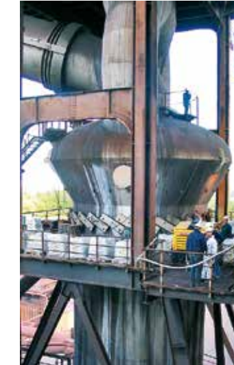
Short lining times for a whirler are achieved with a combined lining of hard compound KALCRET BTS and zirconium corundum KALCOR. The high application rate of KALCRET BTS is 5 m 2 /h
