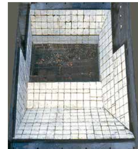
KERAFLEX is a composite material that combines the hardness of KALOCER oxide ceramics with impact resistant rubber
