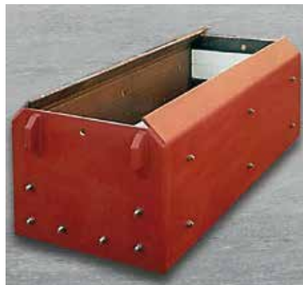
Brake box of a slag granulating system; in the zone of maximum wear the structure of KALMETALL has been lined with KALOCER tiles
