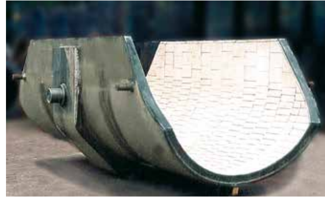
Distributor tilting chute being part of blast furnace lining fitted with KALOCER high-alumina ceramics, 50 mm thick
