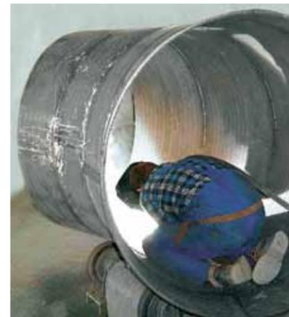
Large diameter dust collection pipes can be cost-effectively manufactured as self-supporting structures of KALMETALL hardoverlay welded plates.
