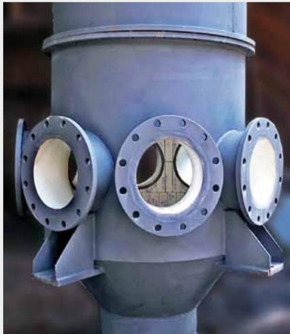
Quite often distributor housings are fitted with rubber lining. Short service cycles suggest ceramic linings: this problem will be solved best with ABRESIST, KALCOR and KALOCER.
