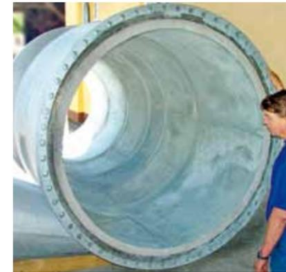
Cyclone lined with KALSICA N silicon carbide ceramics with a diameter of 1,200 mm Ø.
