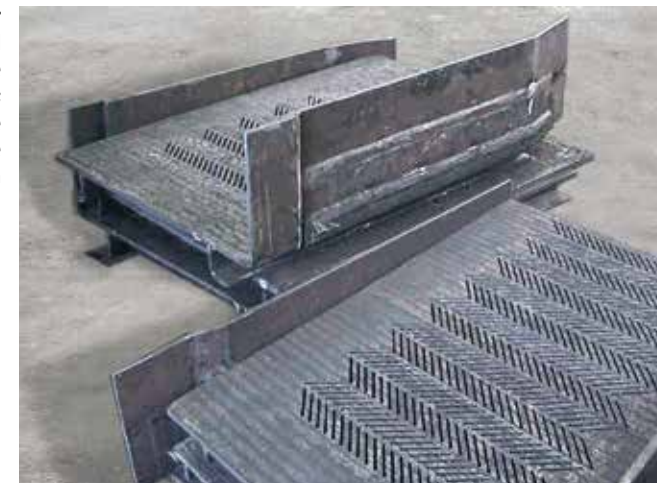
KALCOR zirconium corundum fitted to the deflection zone where abrasive sintered particles impinge at temperatures of 250°C/482°F and high velocity, an economic solution when combined with ABRESIST fused cast basalt
