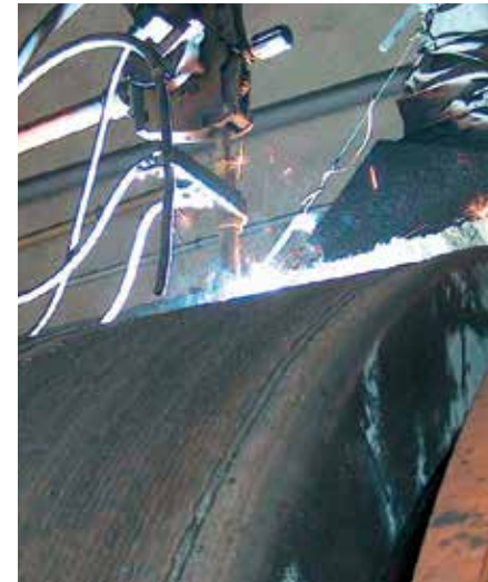
Service by Kalenborn: rebuilding of a grinding roll with KALMETALL W100
