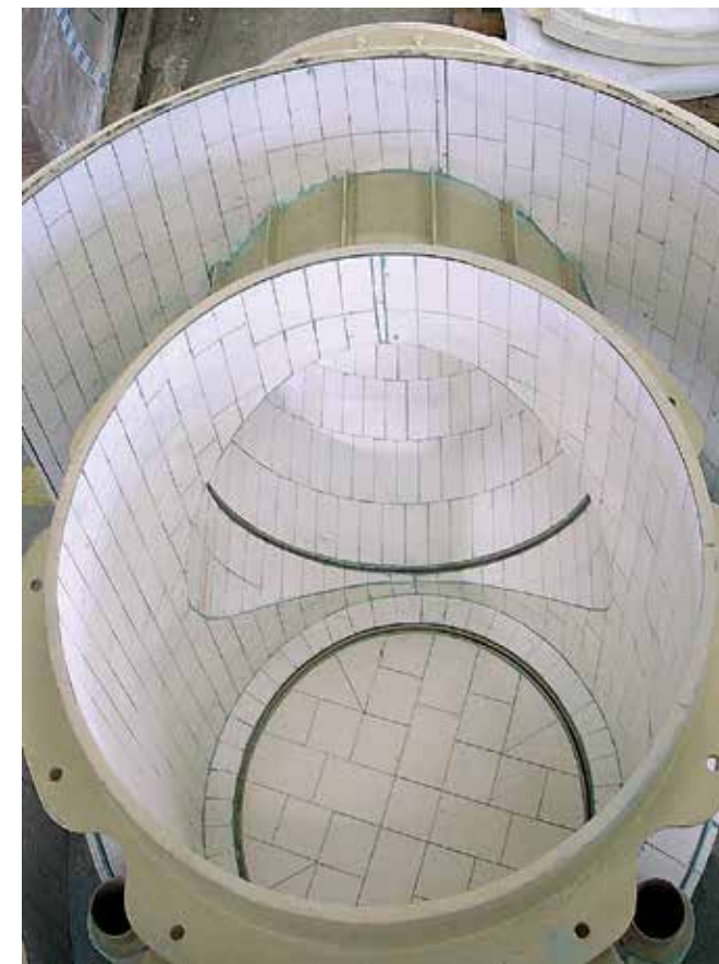
ABRESIST fused cast basalt is a time-tested protective material for cement separators
