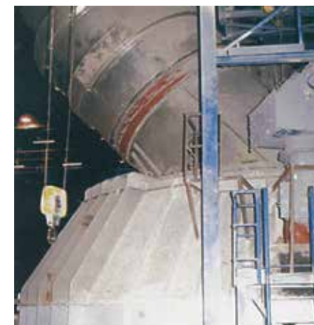
Housing made of KALMETAL for a raw meal fan – 2,000 mm Ø – as segment lining
