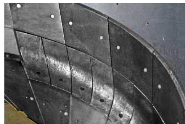
Screens are used in many areas of raw material processing. The herringbone pattern is burned in the KALMETALL hard overlay welded plates.
