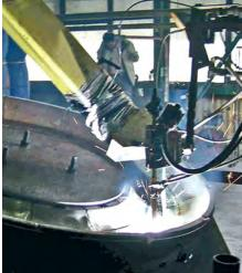
Kalenborn Abresist provides the equipment and expertise to fabricate KALMETALL® chrome carbide weld overlay, standard grades of carbon and AR plate into wear resistant plates, piping and a variety of complete wear protected structures and assemblies. KALMETALL can also be adapted to specific uses by varying the alloy of the hard overlay welding.
