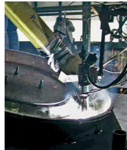
Rebuilding a grinding table with KALMETALL W100.
