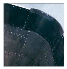
Shaped in a furnace, KALEN linings cut to size adapt themselves to curved surfaces.
