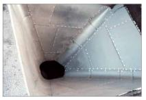
Significant improvements can be achieved by selective measures to reduce wall friction and to avoid adhesion, i.e. by the use of slide promoting linings.
