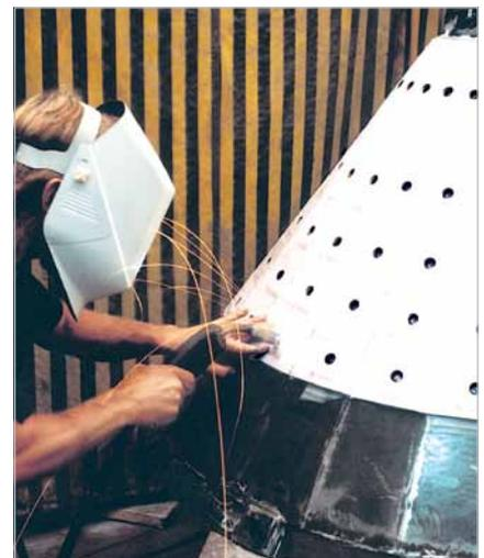
**Mechanically fixed special tiles of KALOCER protect the cone against wear even in case of thermal shock stress**
