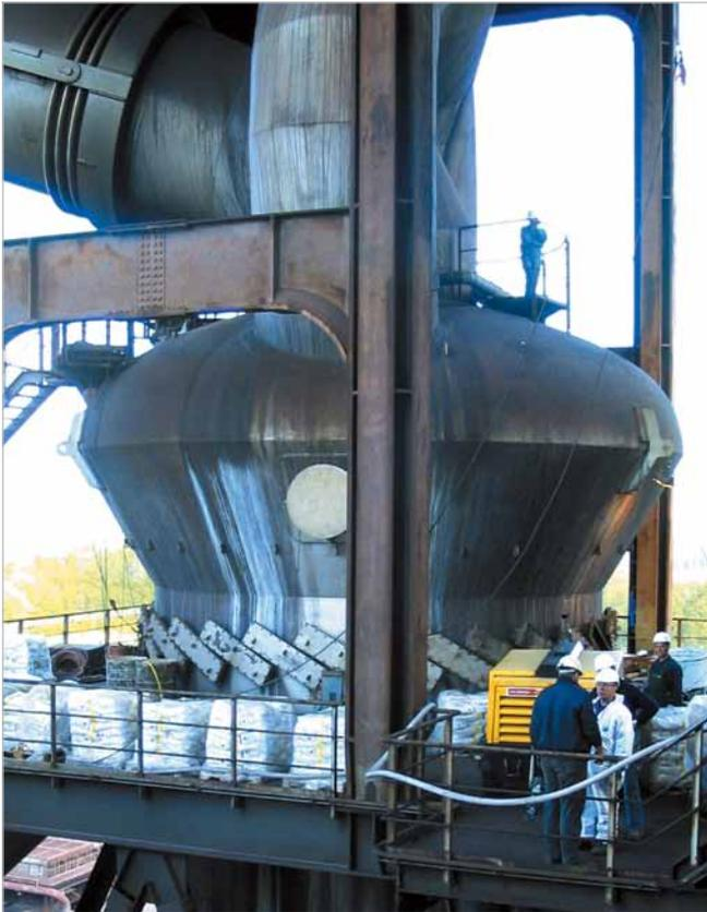
Separator of a cement mill lined with KALCRET-BNX, up to 3,200 mm diameter
