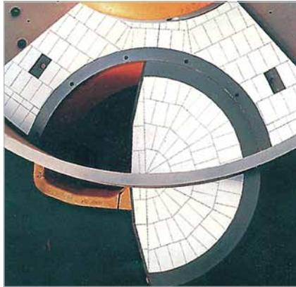
KALOCER bottom of a concrete mixer for extreme stress, KALMETALL-W in the area of the discharge gate
