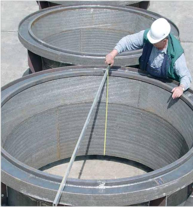
Separating cones of cement classifiers made of KALMETALL-W 100 as self-supporting structures
