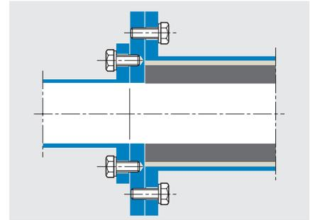
Unlined pipes, pumps or fittings can be connected with a lined pipe using an adapter flange.
