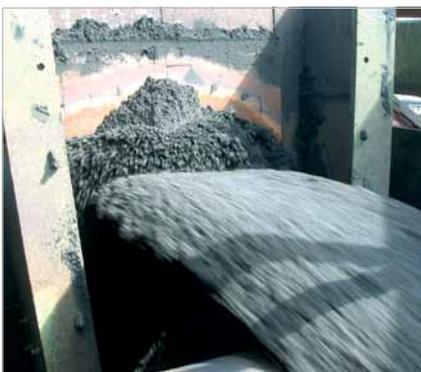
KERFALEX lining of a bin set up in a bulk material handling plant
