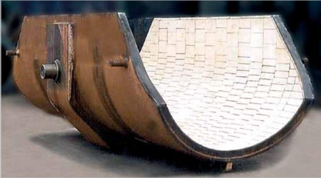
Octagonal hopper in a steel plant; the 50 mm thick
