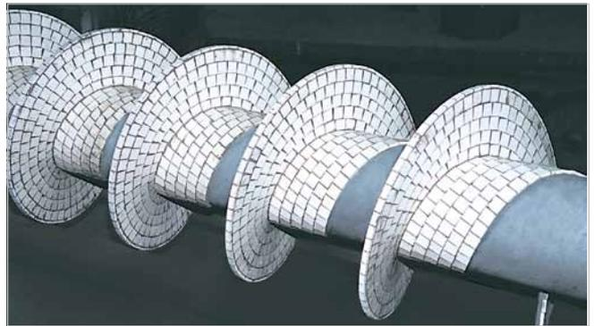
Screw lined with high alumina ceramics
