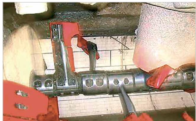
Drum mixer for concrete lined with KALOCER high alumina ceramics; mixer tools made of KALMETALL-C hard casting and/or KALEN-PU plastics
