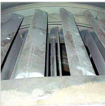
Guide vanes of a separator made
