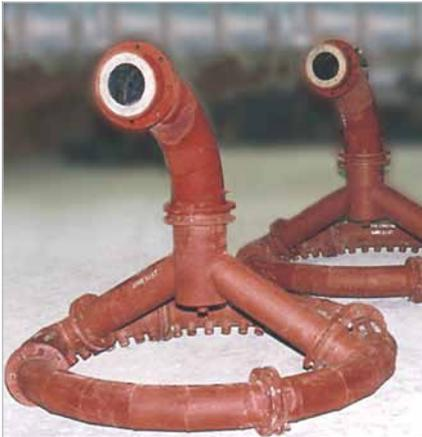
Separator components provided with ABRESIST wear protection
