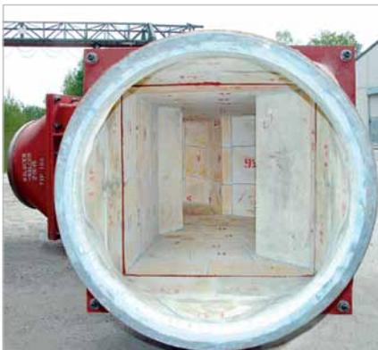
Pulverized coal distributor with reliable KALCOR lining to ensure trouble-free operation
