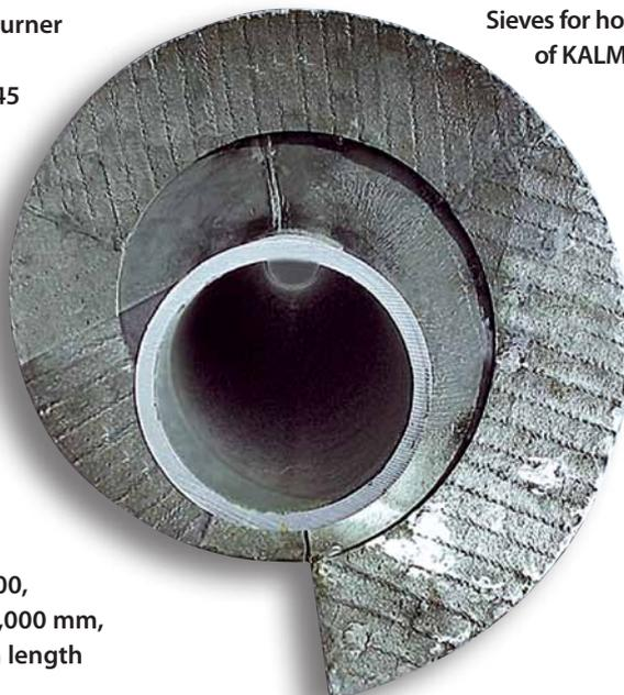
Screw conveyor protected with KALMETALL-W 100, diameter up to 2,000 mm, up to 10,000 mm length
