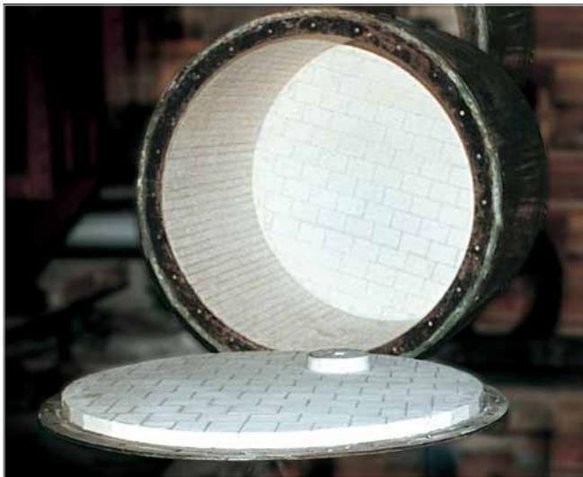
KALOCER lining of a mill for superfine grinding
