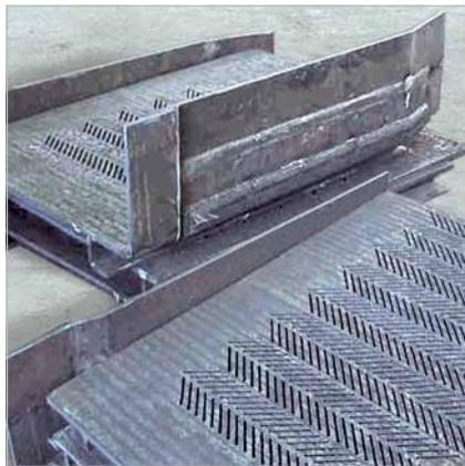
Sieves for hot sinter made of KALMETALL-W 145
