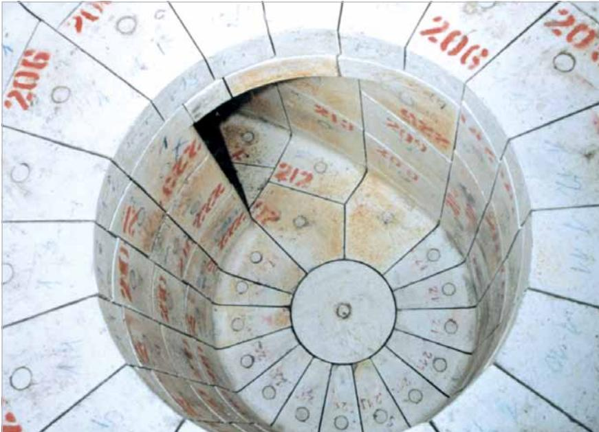
Wear protection for high temperatures involves problems due to thermal stress between the outer steel component and the rigid lining. These problems can be solved by using KALCOR as wear protection material and the right mechanical fixing method: bolted connections or welded steel inserts. Example: drying drum in a chemical plant at 800 °C / 1.472 °F.
