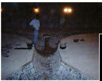
Kalenborn Abresist flume linings have been engineered, designed and installed in a rolling mill and in continuous caster flumes for many years. Most are still performing as well as the first day with minor repairs caused by dropping large objects into the flumes.
