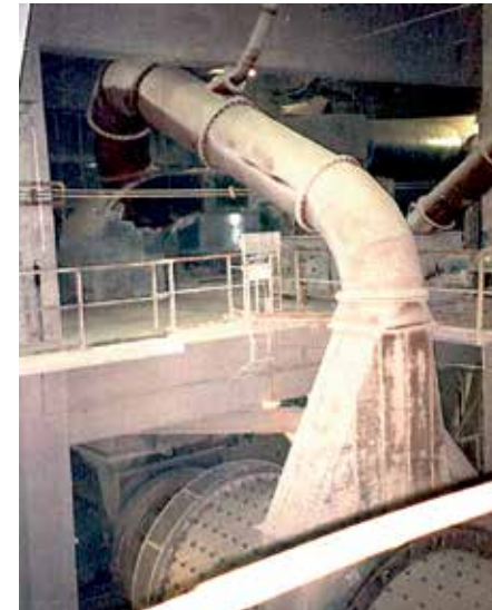
ABRESIST used for the center discharge duct of a ball mill
