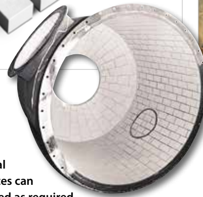
Chutes lined with KALCERAM are a solution that lasts, e.g. for bag loading systems in cement plants
