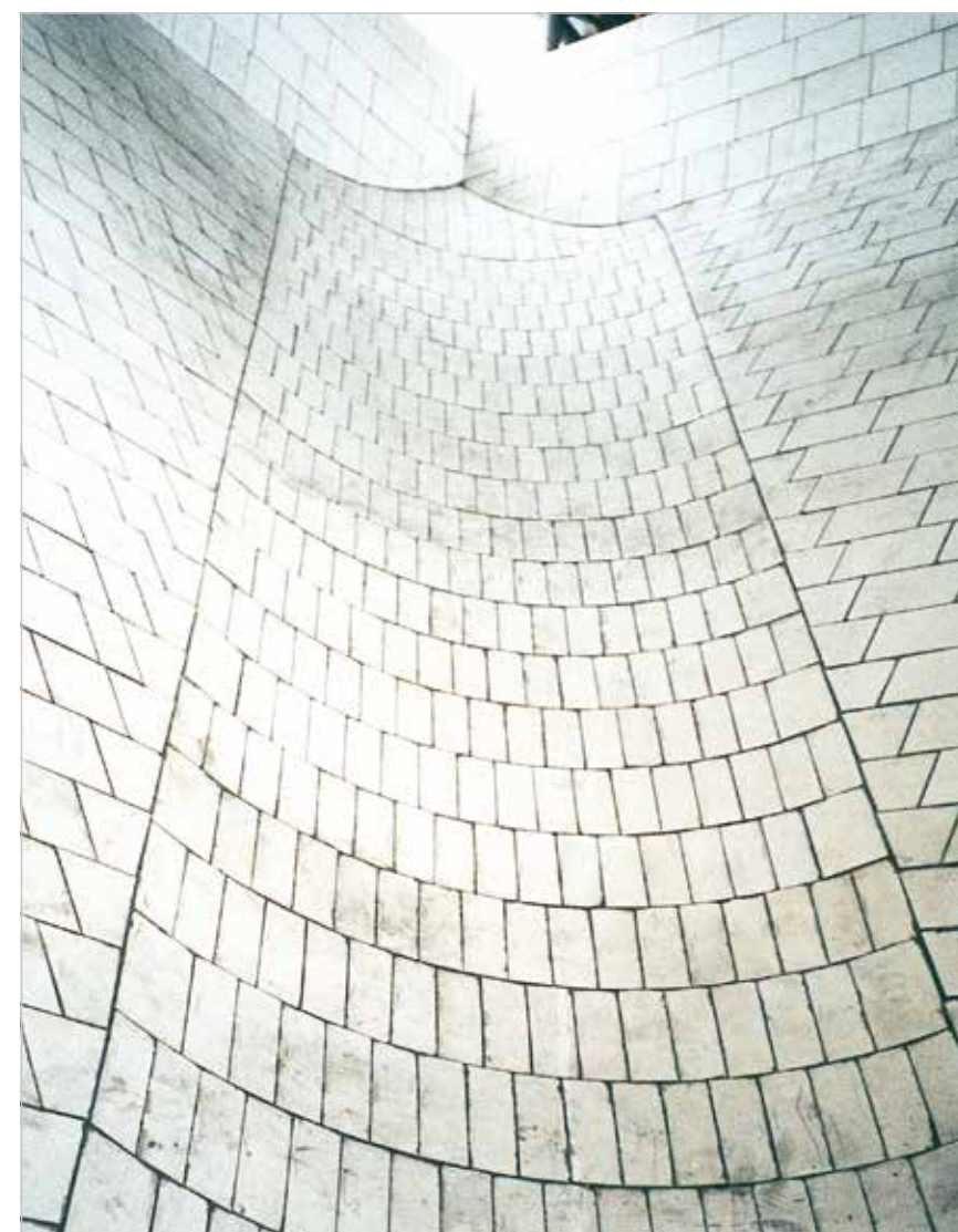
Skip collection chute with KALOCER lining installed at a European blast furnace plant; the shaped elements are up to 50 mm thick and have been cut three-dimensionally to fit the component.
