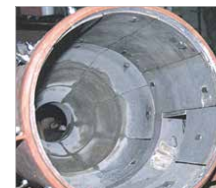
Cyclone used in a soil decontamination system – effectively protected with KALCAST
