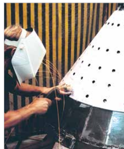
Mechanically fixed special tiles of KALOCER protect the cone against wear even in case of thermal shock stress
