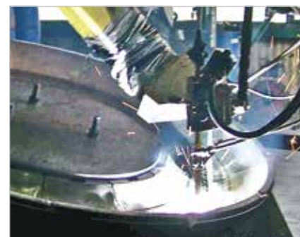
Kalenborn welding service, regeneration of a grinding table
