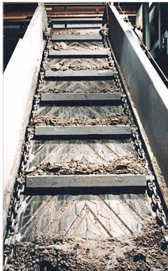
Chain conveyor for wet ash removal in a power plant. Drains cast into the lining reduce the undesired carrying of water to the discharge zone thereby lowering the water consumption rate.
