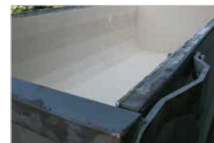
Seamless lining of a dump truck bed
