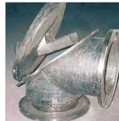
Pulverized coal burner lined with KALMETALL
