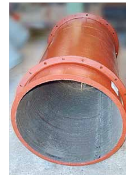
Pipe armored with KALMETALL installed in a dust collecting system; inside diameter 400 mm, system thickness 8 + 5 mm
