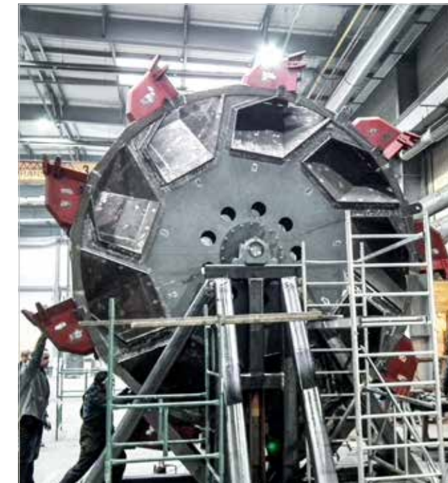
For a steel manufacturer in North Africa, a bucket wheel as a custom KALMETALL welded construction
