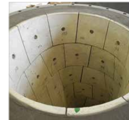
Convex dryer inlet with KALCOR-lined tiles
