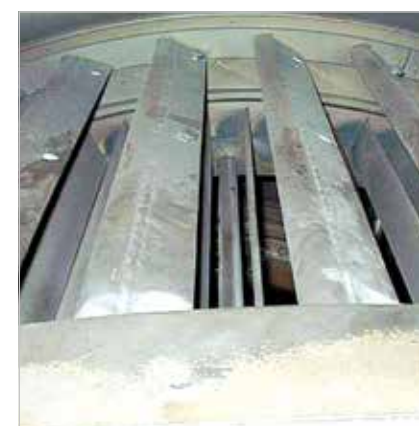
Guide vanes of a separator made of KALSICA operated within a coal pulverizer
