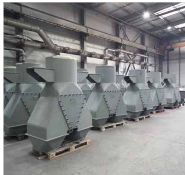
Pulverized coal distributors made of KALMETALL
