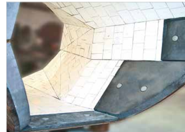
Octagonal hopper subjected to impact stress lined with three-dimensionally cut KALOCER shaped elements as well as KALCAST shapes, each 50 mm thick
