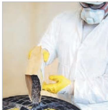
2.2 Add fiber components slowly and continuously and mix dry for at least 1 minute
