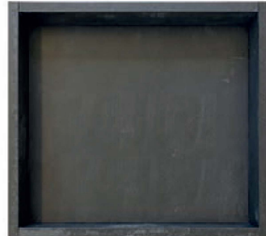
Plastic sample form: 320 x 300 x 40 mm
