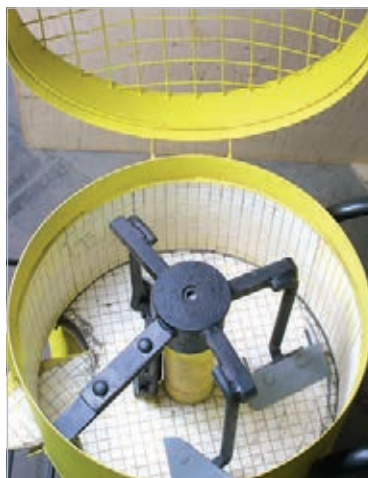
Wear protected tank of a Kalenborn forced circulation mixer
